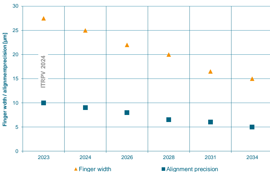
Fig. 32: Predicted trend for finger width and alignment precision in screen-printing. Finger width needs to be reduced without any significant reduction in conductivity.
